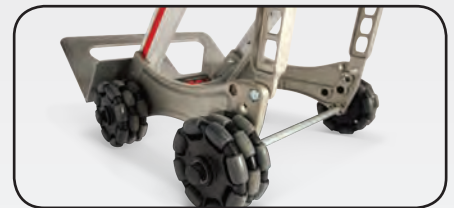
Wheelbase: 4xRC Rotacaster/R3
