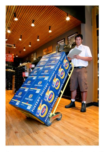
Photo: Rotatruck Self Supporting Hand Truck. Note that the parked load is fully supported and permits the operator's hands to be free to conduct administrative tasks.
